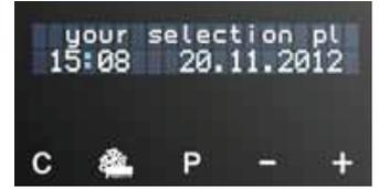
The 1200S keeps it simple with all important functions & operations easily accessible and editable using a two line display and 5 function keys.
